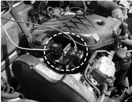
Fig. 3. ADXL sensors on engine block
