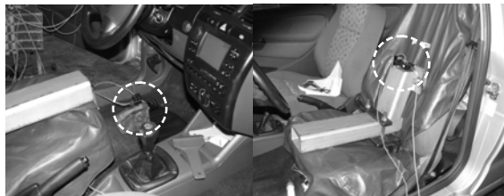
Fig. 4. ADXL sensors on floor panel and seat
